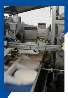
To transport product from the lidding machines through a metal detector, checkweigher and proceed onto a packing station conveyor prior to cartoning
